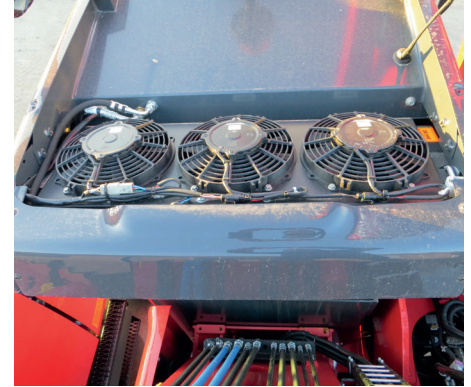
3 air conditioning fans separated from the main radiator for a more efficient cooling system.
