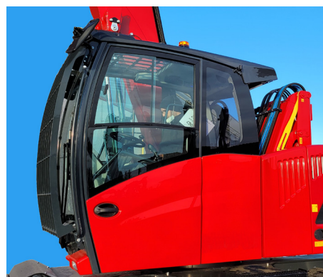
Driver's cab with large glass surfaces and left sliding side window.
