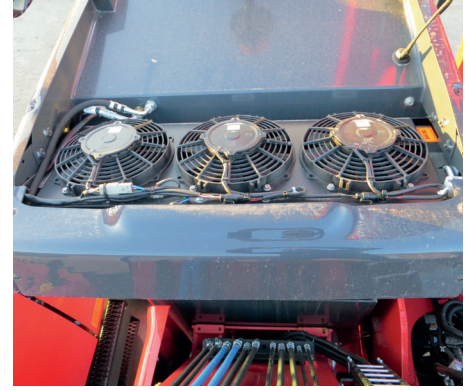
3 air conditioning fans separated from the main radiators for a more efficient cooling system.
