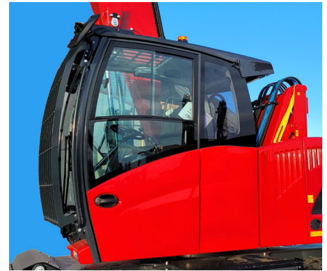
Driver's cab with large glass surfaces and left sliding side window.
